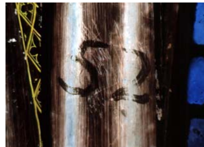
fig. 21 Scratch marks in glass paint
