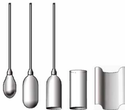
fig.77 The different stages of cylinder glass production
