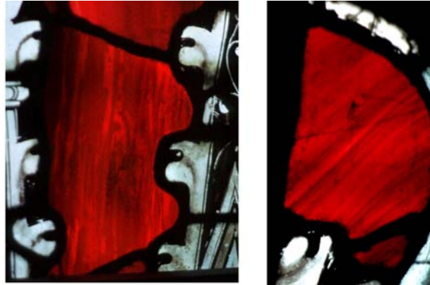
fig. 20 Etched (left) and real (right) streaky ruby glass
